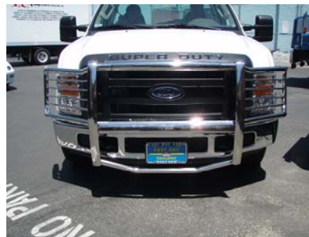
Fully assembled & installed brush guard.
