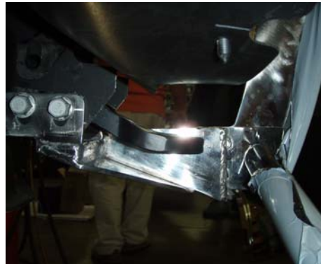
Bracket with 2 bolts on passenger side and bottom bar shown.
