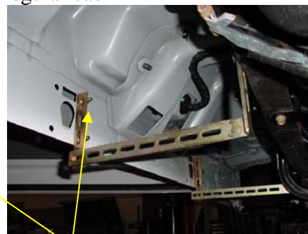
Bracket #4 is mounted to the existing factory holes shown here.
