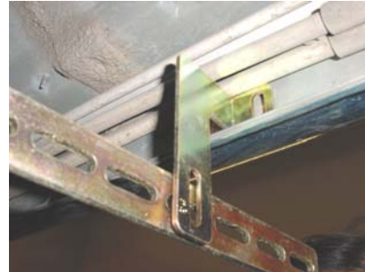
Passenger side shown above. Note: Use extreme caution when pushing the A/C lines upward to gain clearance.
