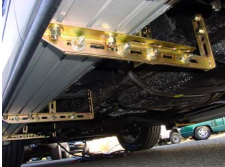
Driver side brackets config shown for 2001 ML320.
