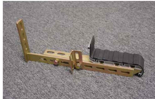
Configuration to mount on outside pinch weld.
