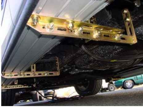
Driver side brackets config shown for 2001 ML320.
