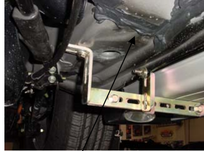
Optional: Driver side rear using #1,2,5. bent bracket and mounted to the floor.
