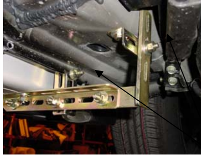
Passenger side rear using #1,2 and 2 #5 brackets, Note: shorten bracket #2 by 1" to clear.
