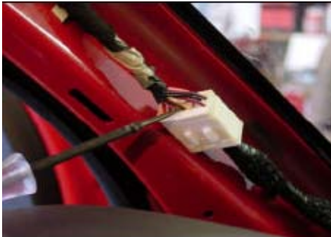
Dome light wire is on driver side pillar, Brown (- trigger).
